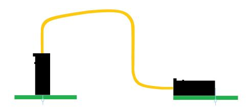
The flexible jumper cable can also have one end of the pins connected to this connector, while the other end of the pins is soldered through holes on the circuit board.
